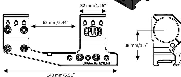
The mounts are machined from billet 7000-series aluminum and all aluminum parts are hardcoat anodized. The Torx 20 ring and clamping screws are zinc-nickel coated for corrosion resistance and come pre-waxed from the factory to ensure proper torque values.
