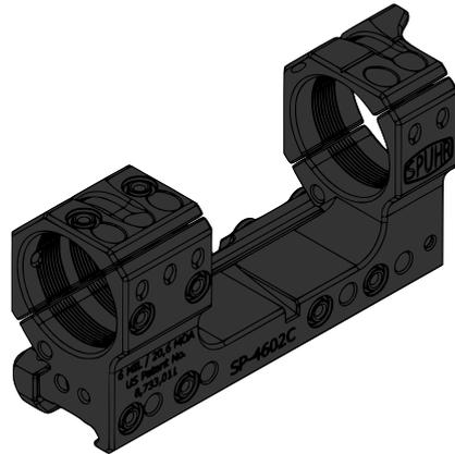
The **IDEAL SCOPE MOUNT SYSTEM** series of mounts feature **seven set of interfaces to attach any of more than 40 different accessories** and has a bubble level integrated in the rear plane of the mount body to prevent canting of the rifle. The rings are diagonally cut for increased visibility of the elevation and windage turrets (US Patent 8,733,011).
