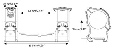
The SCP-3001D Interface Mount features two Spuhr Interface™ Top Covers, which can be installed as to position any of more than 40 different accessories in either the 12 or 3 o'clock position.
